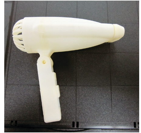
3D printed hair dryer produced by students to test the functionality of the grip
