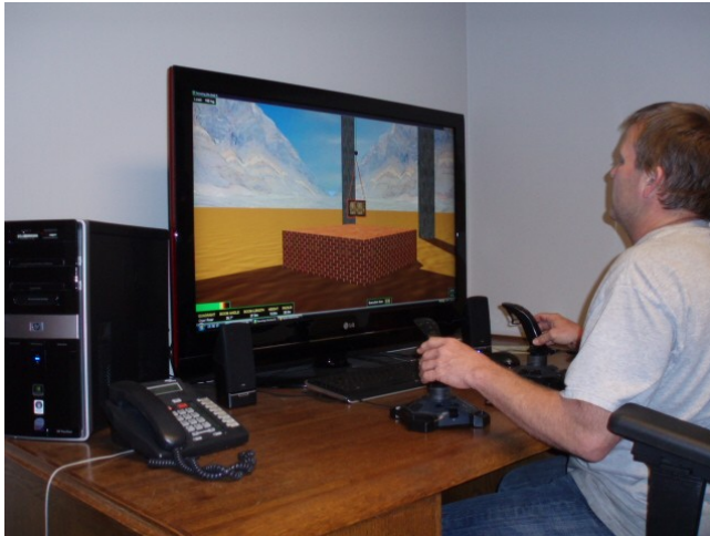
A single PC with Simlog's Hydraulic Excavator, Tower Crane and Mobile Crane simulators sharing the same PC Controls at Local 701's Gladstone headquarters.
