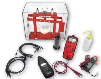
Industrial Loads with Prony Brake
