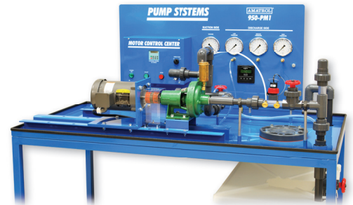
Centrifugal Pump on the 950-PM1
